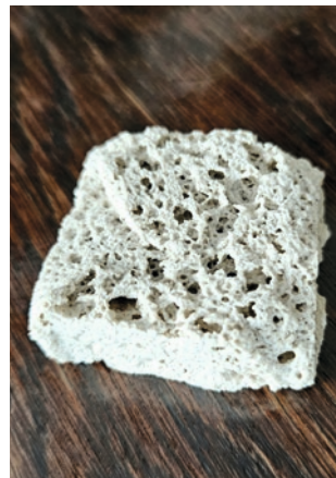
Figure 2: Solidified biogenic "porestone".
